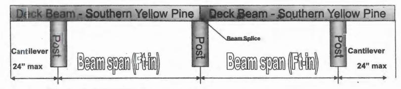
DECK BEAMS - SOUTHERN YELLOW PINE #2 - simple span joist
