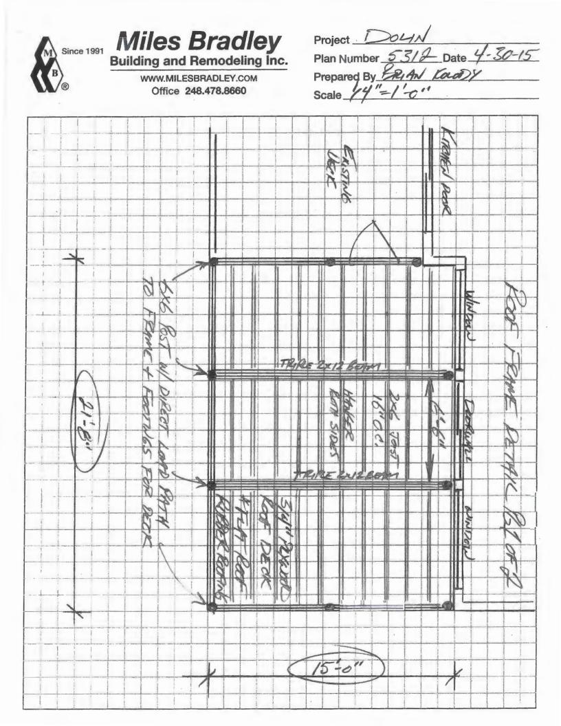
Project DOUA Since 1991 Miles Bradley Plan Number 5312 Date 4-30-15 Prepared By BRIAN Kocorry Building and Remodeling Inc. WWW.MILESBRADLEY.COM Office 248.478.8660 Scale NOT TO SCALE RUBBER (EPDM) MEMBRANE RUBBER ROOF UNDERLAYMENT 3/4 "PLYWROT ROOF DECK 2×6 CEILAKS JOIST 246 Tast HANGERS FINISTED TTO CEILING" COFFERED" STYLE TRIPLE 2×12 Roof BEAMS JRAP BOTTOM OF EMIS WITH IK SPF OF FRAME DETAIL
