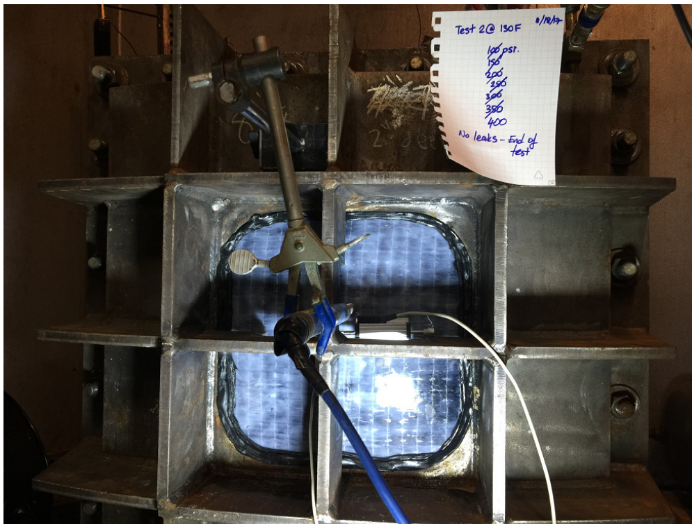
Figure C.6 – View of Specimen 130F-2 at termination of test (404 psi, no leaks).
