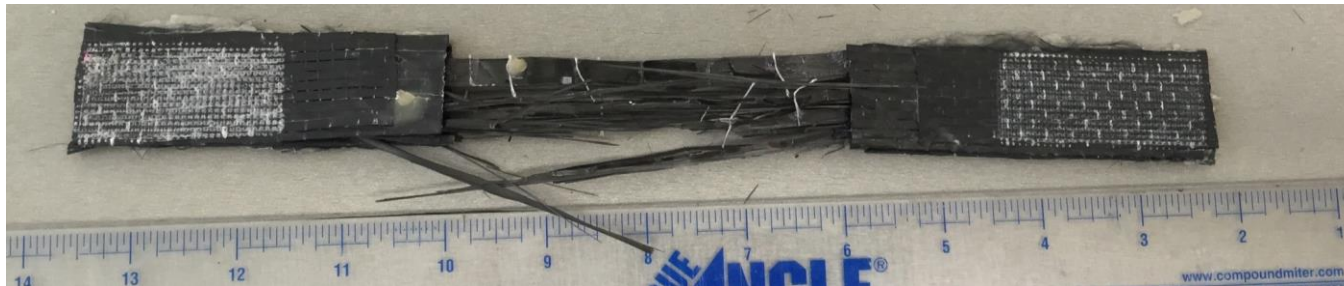
Figure 1.2 – Representative failure mode XGV: eXplosive, at Gage, in the Various locations
