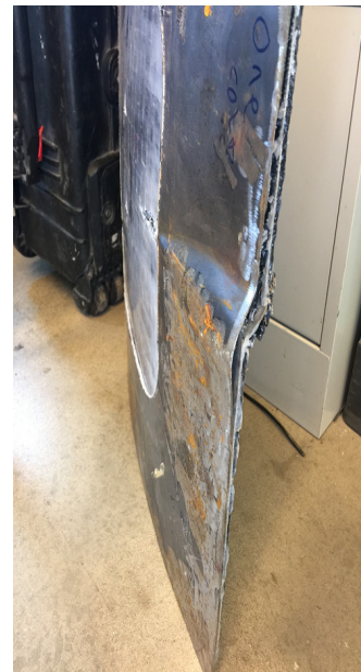
Figure C.1 – View of Specimen 32F-1, (a) at termination of test at 345 psi, and (b) edge of specimen after removal from pressure chamber. (Note that the failure was due to local bending of the specimen at the seating tabs within the chamber, and not due to the performance of the laminate architecture.)
