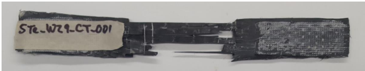
Figure 1.2 – Representative failure mode, M(S,A)GM, Multiple (Longitudinal Splitting and Angled), at Gage, in the Middle
