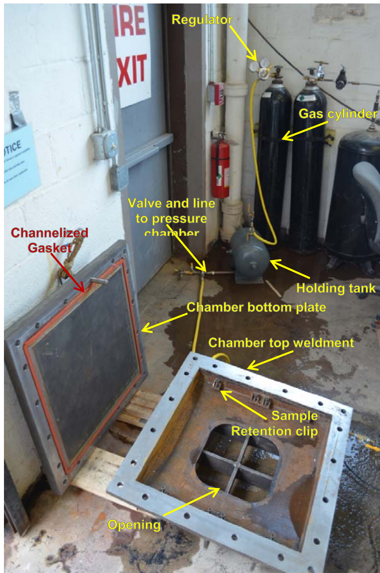
Photo 1 – Test apparatus disassembled (left) and assembled (right).
