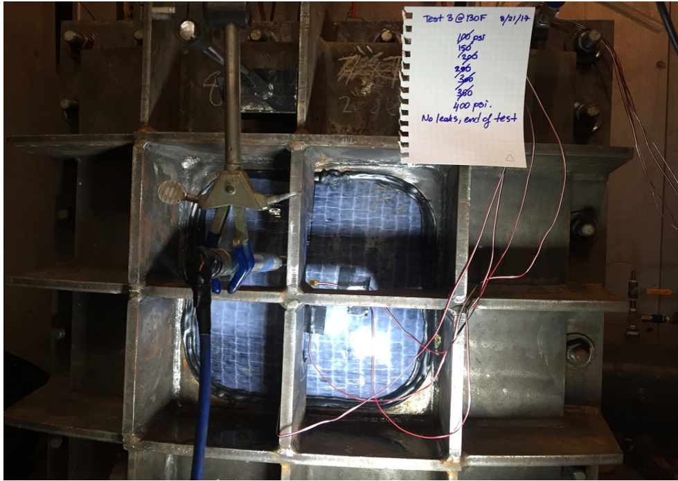
Figure C.7 – View of Specimen 130F-3 at termination of test (402 psi, no leaks).
