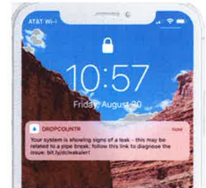
LEAK ALERT VIA PUSH MESSAGE
