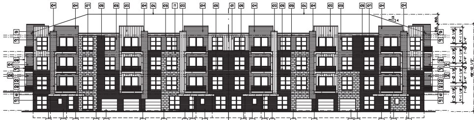
REAR ELEVATION BUILDING 250 BUILDINGS WILL STEP TO FOLLOW FINAL GRADE - SEE CIVIL DRAWINGS SCALE: 1/16" = 1'-0"
