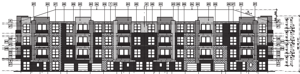
REAR ELEVATION BUILDING 255 SIMILAR TO BLDG. 250 BUILDINGS WILL STEP TO FOLLOW FINAL GRADE - SEE CIVIL DRAWINGS SCALE: 1/16" = 1'-0"
