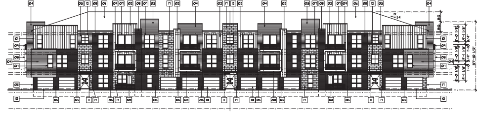
FRONT ELEVATION BUILDING 250 BUILDINGS WILL STEP TO FOLLOW FINAL GRADE - SEE CIVIL DRAWINGS SCALE: 1/16" = 1'-0"
