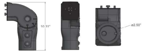
SF - Slip Fitter Arm Dimensions
