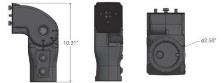
SF - Slip Fitter Arm Dimensions
