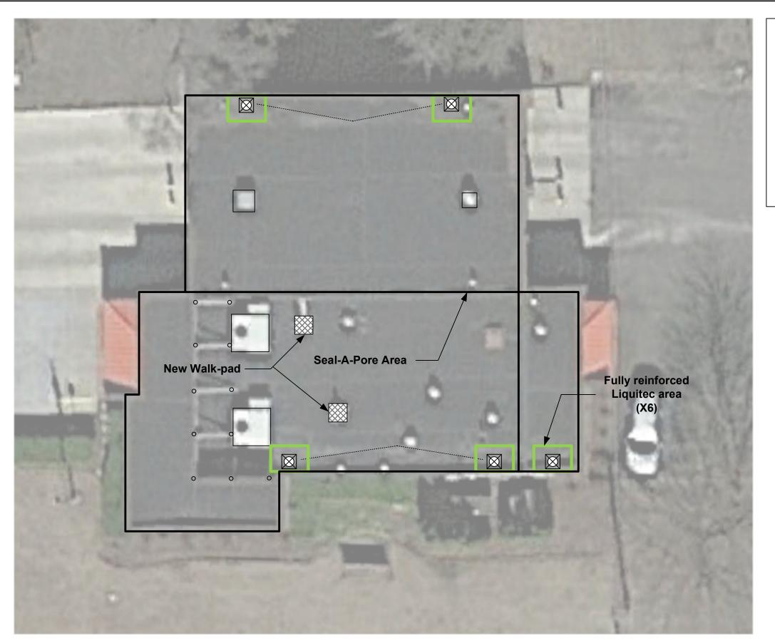
Seal-A-Pore Area: Apply Sealant to masonry wall at elevation change: Caulk control joint
