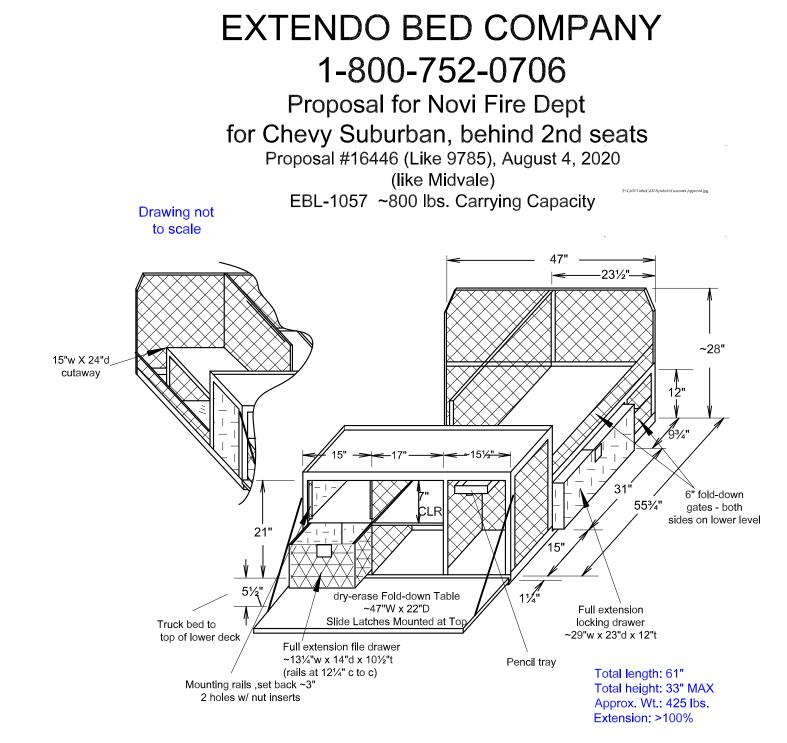
Platforms will be 1/2" OSB Superstratum. Carrier will be built of 1-1/4" by 1/8" steel angle, & with 1-1/2", 10 gauge flattened steel mesh material. Aluminum drawers and exterior panel will be of .080 diamond plate aluminum. Inside panels & shelves of cabinet will be .100/.125 smooth aluminum. Fold-down table is of polypropylene, in steel frames.
