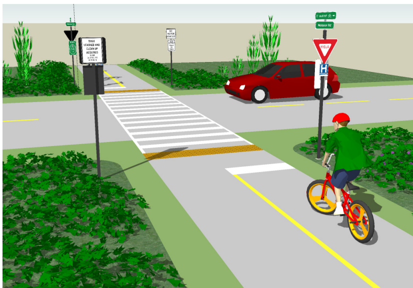
Fig. 5.11C. Trail Signs at Road Intersections Trail View
