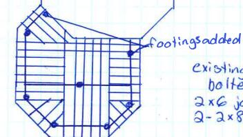
existing deck GxG footings notched currently lag bolted. To be carniage bolted 2xG joists doubled/hangered 160.c. 15" cantelier 2-2×8 Beams
