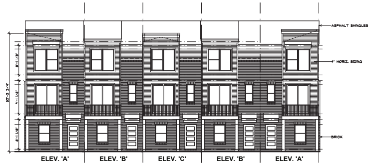
FRONT ELEVATION 5 UNIT BUILDING
