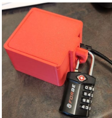
Mary designed and 3D printed an "Electrical Plug Lockbox" for use in the iCube. The box prevents unauthorized use of equipment by preventing it from being plugged in.
