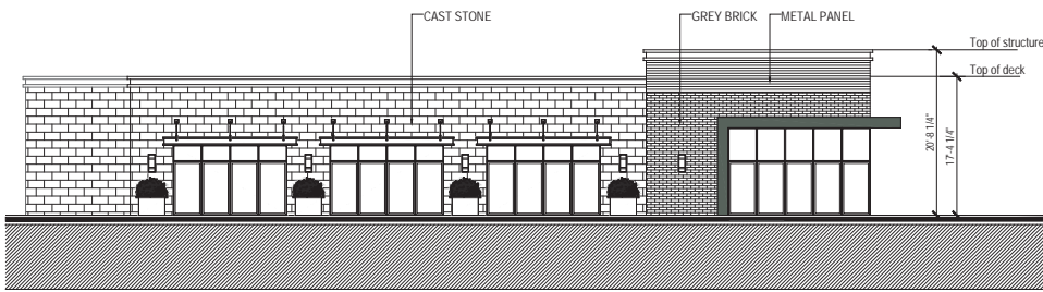
SIDE ELEVATION BRICK 17% CAST STONE 74% METAL PANEL 9%
