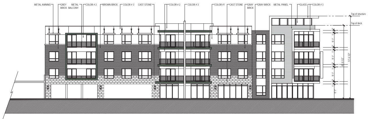
SIDE ELEVATION ( South/ pool courtyard)
