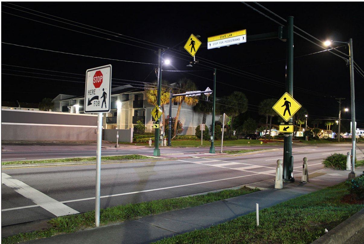
Signage and pavement markings can be highly effective in improving safety for vulnerable road users. Source: FHWA
