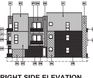
RIGHT SIDE ELEVATION BLDG 100 SCALE: 1/16" = 1'-0"
