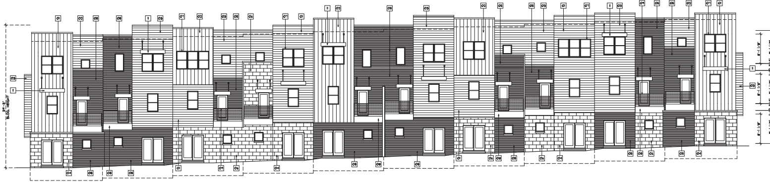
REAR ELEVATION NOTE: BUILDINGS WILL STEP TO FOLLOW FINAL GRADE - SEE CIVIL DRAWINGS
