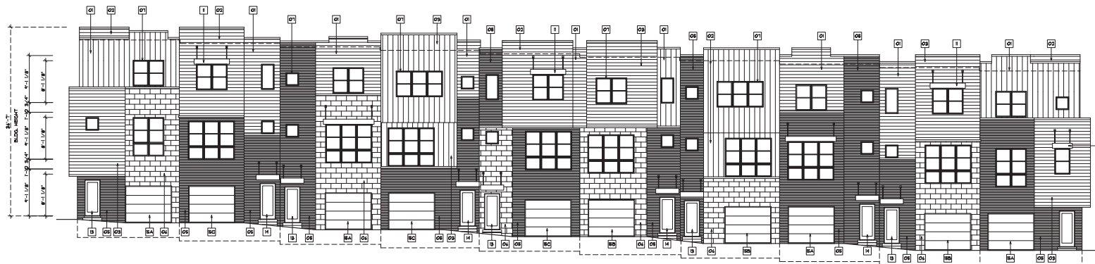
FRONT ELEVATION NOTE: BUILDINGS WILL STEP TO FOLLOW FINAL GRADE - SEE CIVIL DRAWINGS
