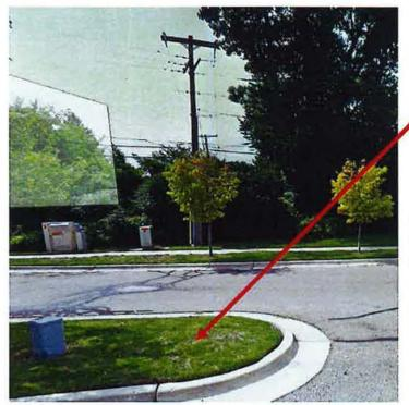
City of Novi is requesting a Code 16A with an 80W LED Acorn to be Installed on the north end of Blvd on Bethany Way, North of 10 Mile. Will need to feed the light from the wood pole on the West side of road
