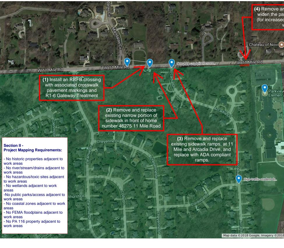
(4) Remove and replace existing damaged pavement and widen the paved area for the turn south into the school (for increased visibility and more turning room for users with bicycles and wheelchairs) Taft Rd
