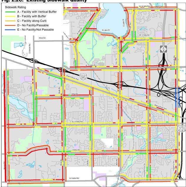
A key factor to a pedestrians comfort on a sidewalk is the degree of separation from the roadway. Buffer (lawn extensions) and vertical elements such as trees and light poles increase the pedestrians comfort level.
