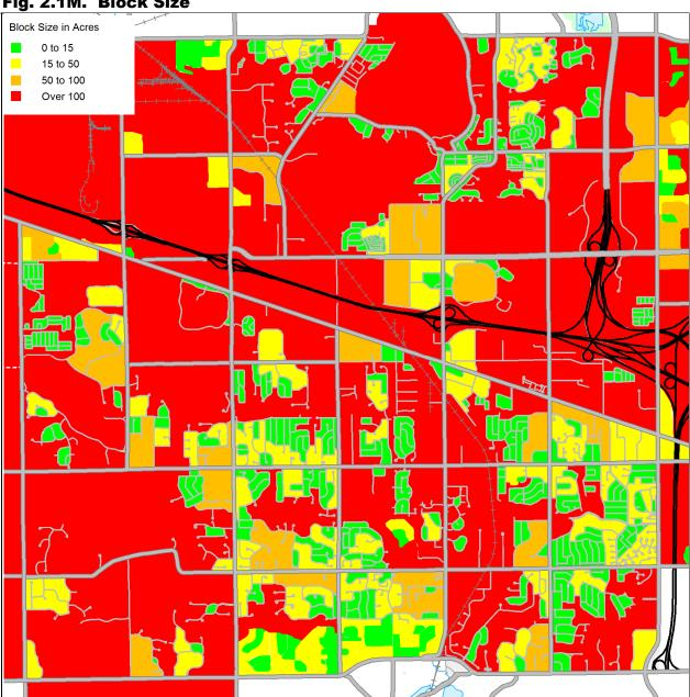
Block size is an excellent measurement of directness of travel and a key indicator in the level of pedestrian activity. A block is defined as an area that a person cannot pass through. These areas usually do not have any sidewalks, roadways or bike paths allowing access between two points. One example is an expressway where you may have to go a mile or more out of your way just to get to the other side.
