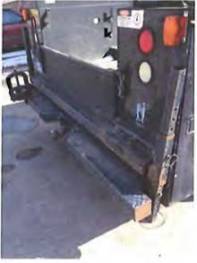
The point of egress on a service truck is the rear bumper and tailgate assembly. The current service truck bumper is suffering from corrosion and has had the external stabilizers serviced multiple times due to this. The new service truck will have a formed step platform for egress as well as an incorporated storage compartment for long tools.
