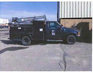
The service truck capacities should reflect the capacities required in the field operations. The current service truck is based on an F350 chassis, and lacks the towing capacity for the Water and Sewer Division's excavating equipment. The new service truck will have increased capacities to efficiently operate in the field.
