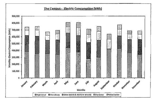
The average electric demand for the Campus is approximately 1,000 kW and sufficient thermal loads exist within the campus to support a 1 MW base load CHP facility. Prime mover for the CHP facility is assumed to be a 1 MW reciprocating engine generator, and
