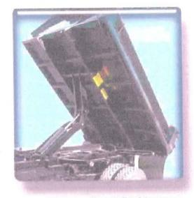
The Yardbird features a fully-interlaced subframe, full depth corner posts, as well as fullyenclosed front corner posts. The Yardbird's heavy duty platform hinge is greaseable.
