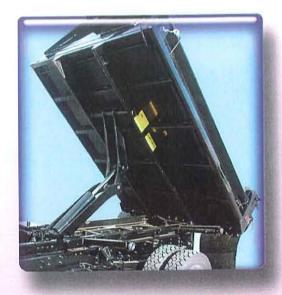
The Yardbird features a fully-interlaced subframe, full depth corner posts, as well as fullyenclosed front corner posts. The Yardbird's heavy duty platform hinge is greaseable.
