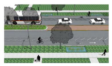
Where space permits, a painted buffer zone should be incorporated between the bike lane and the motor vehicle lane for added safety and separation from vehicles. Flexible posts may also be included as to increase bicyclists comfort.
